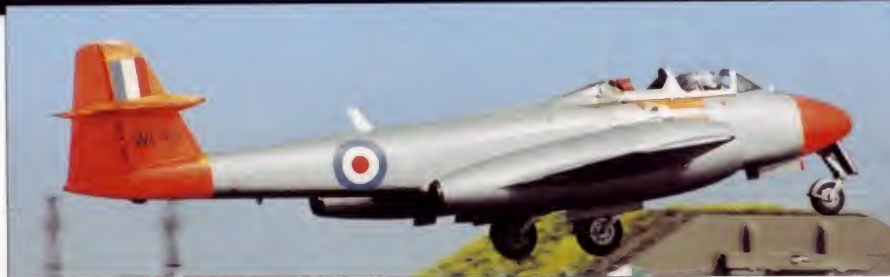
The high-set, conventional tailplane was typical of the 'low-risk', conservative approach to the Meteor's design.
